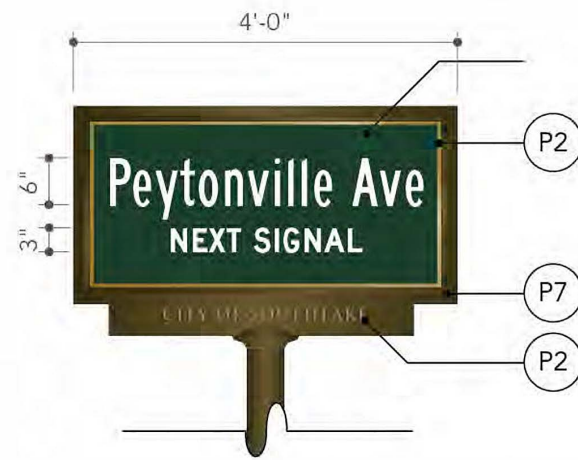
6 Alternative Sign Sizing - 48" Width Scale: 1/2" = 1' - 0"
