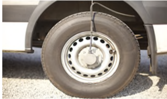
Figure 20: Distance Measuring Instrument (DMI)
