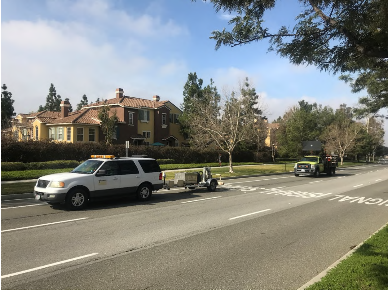
Figure 15: FWD Testing along City Arterial Roadway
