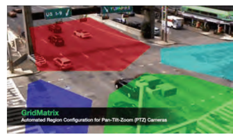
Figure 6: GridMatrix’s software identifies the camera is in its original position and resumes collecting data on congestion and other metrics
