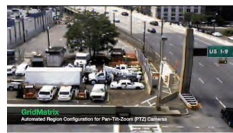
Figure 6: GridMatrix’s software identifies the camera is in its original position and resumes collecting data on congestion and other metrics
